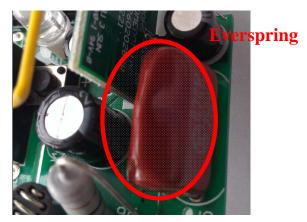
TKB use "Power integrations" power on/off chips, isolation power is safety for people, current output is stable. The power consumption is about 0.5w with energized. It is accord with the EU regulations
