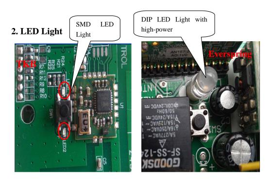
**TKBHOME TZ68** use 3.3 V SMD LED with Lower power consumption **Everspring AN157-7** use DIP LED with higher power consumption.
