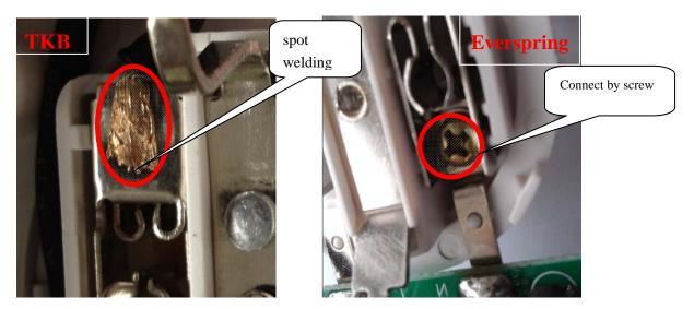
**TKBHOME TZ68** use spot welding to connect the wires, when the products connect to heavy load, it's more safe if the temperature of touch point is lower.
