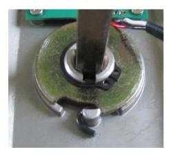
If handle is on the left hand side (seen from outer door side) Place the spring and the metal plate like below
